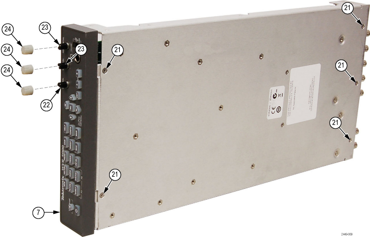
Figure 14: Front Panel assembly removal
